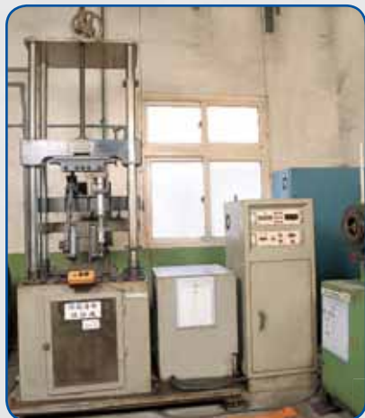
Test durata Life Testing (Reciprocating)
